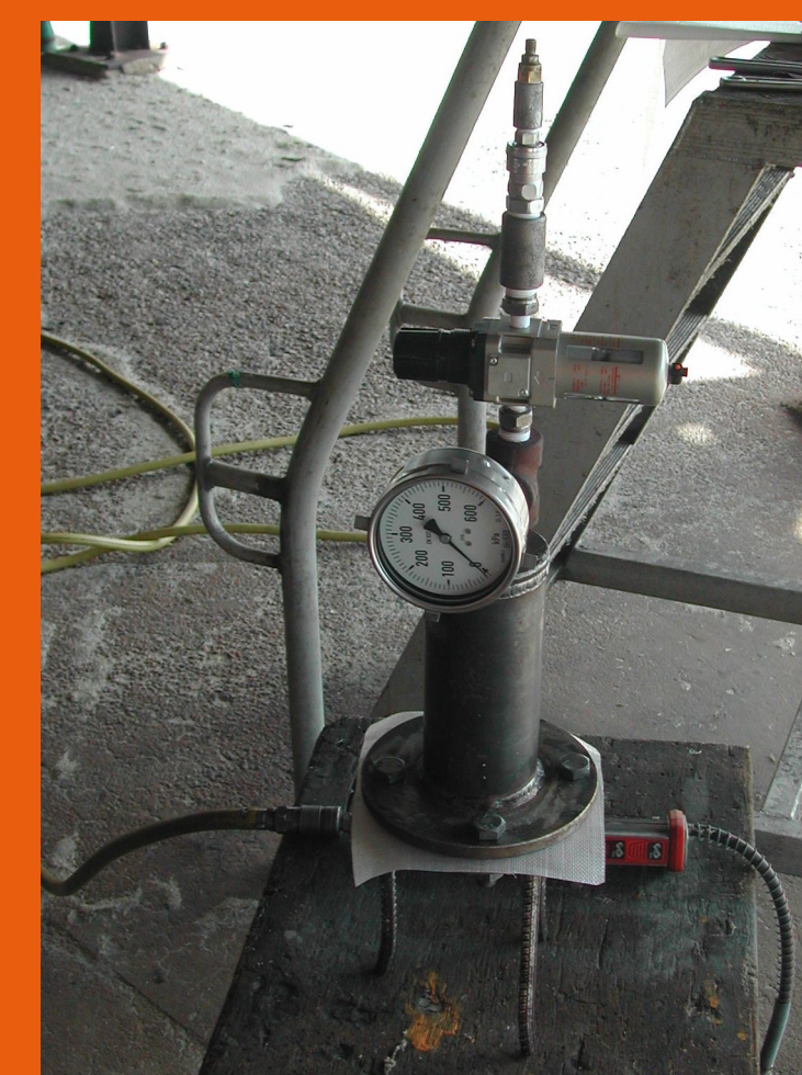
No galvanised fittings are permitted to be used on this apparatus
